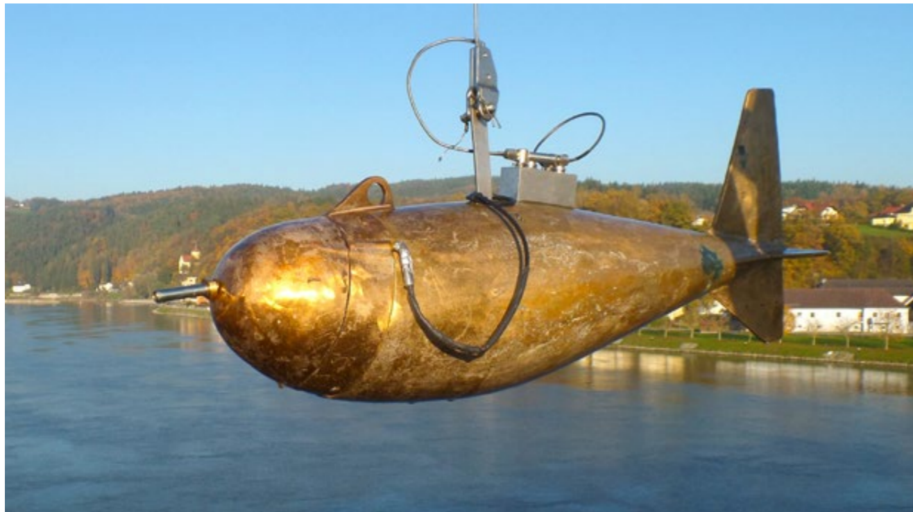
The two photos show instruments used to monitor sediment. The top photo shows a US P63-Sampler, which is a best practice device for monitoring sediment. The photo directly above shows a water sampling method used to analyse suspended sediment
