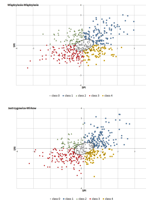
Fig. 5. The SPI vs. SRI correlation plots for the coupled meteorological and hydrological stations for a) Nysa Kłodzka and b) Proсна study basin
